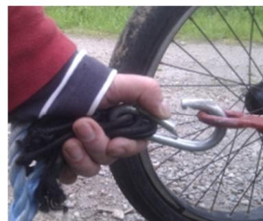
5. Pass the tow rope to the rear of the cartie and attach the top rope through the rear tow rope guide. Note that this is NOT load bearing – it is only to keep the rope centralised so it does not foul on the cartie wheels when going around corners.
